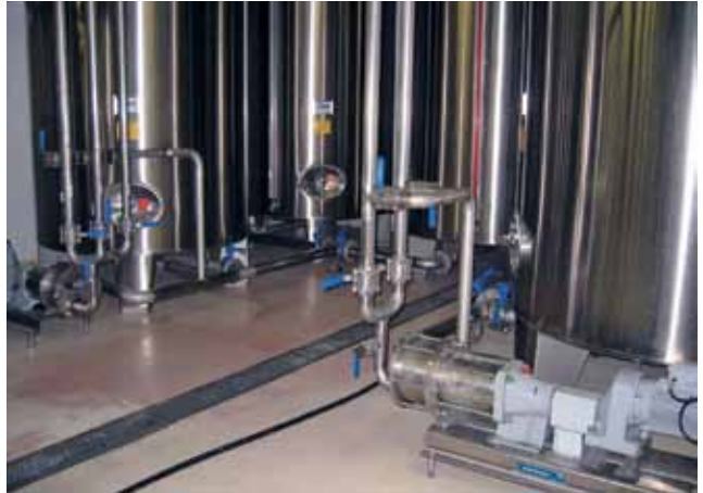
This eccentric disc pump in a hygienic application provides consistent performance that does not change over time.
